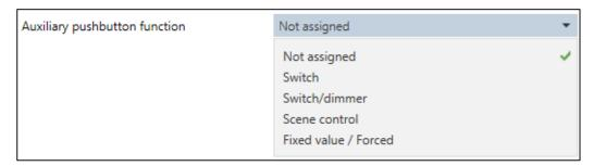
This Actuator can be controlled locally through a wired pushbutton. It is possible to assign different functions, each of which will activate different objects.
