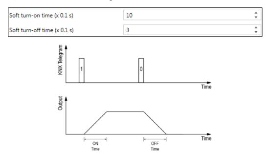
**Dimming Value Fade Time:** fade time when receiving a dimming value.
