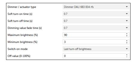
**Soft Turn-On/Off Time:** it allows soft switching on / off, in a fixed time.
