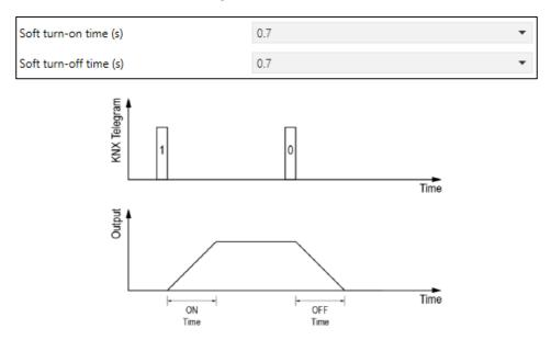
**Dimming Value Fade Time:** fade time when receiving a dimming value.
