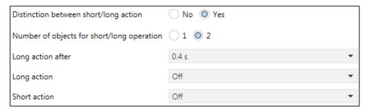
In this case, it is possible to select whether to act on a single object (Number 11 – Switch On-Off Output Short operation) or on 2 different objects (Number 11 - Switch On-Off Output Short operation and Number 12 - Switch On-Off Output Long operation).
