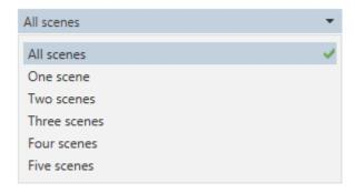
Each of the scenes can be configured with ON or OFF and the desired Scene can be activated through object "Number 4 – Scene Numbered Input".
