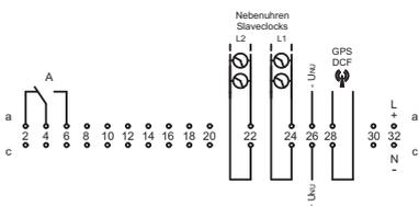
2 slave-clock-lines. Line 2 can be separately configured to pulse every minute or second
