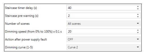
**Staircase Timer Function:** it allows adjusting the timing and the pre-warning time of the Staircase Lighting Timer function (optional). This timing is activated through the object "Number 6 - Timed Start-Stop Input". Each time a "1" is received on that object, the time is reset and the timing starts again.
